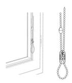
APPLY ONE HALF OF THE COUPLER TO EACH END OF THE CHAIN AND THEN LOCK BOTH COUPLER HALVES.
