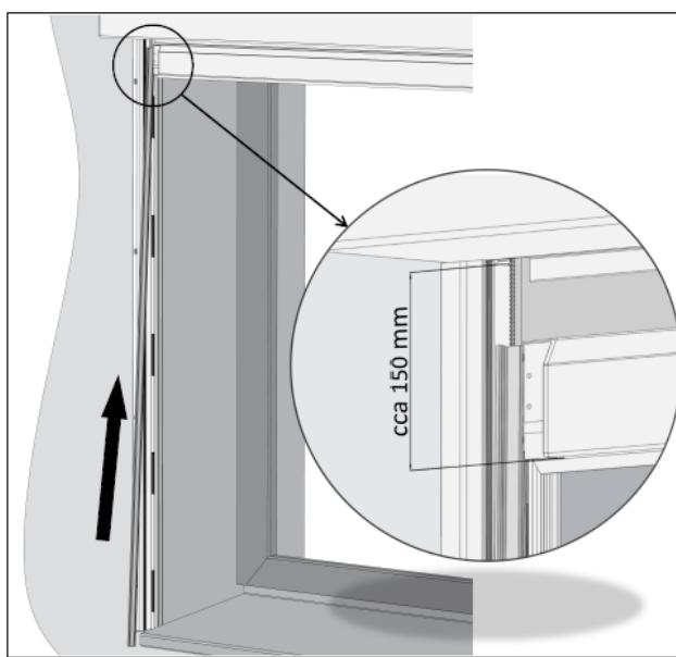
**Sezione guida A840-1 dopo l'inserimento del profilo a zip**
